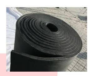
IP Flex flexible elastomeric foam rubber insulation is closed cell construction and features low thermal conductivity and superior temperature resistance, Class 0 fire index, non-hygroscopic, shockproof and sound absorptive. IP Flex is fibre, formaldehyde and ozone-depletion free and poses no health risks. The insulation is supplied in either sheet and pipe form, widely applied in HVAC applications, ductwork, hot and cold water lines, mining pipeline systems and refrigeration applications.
